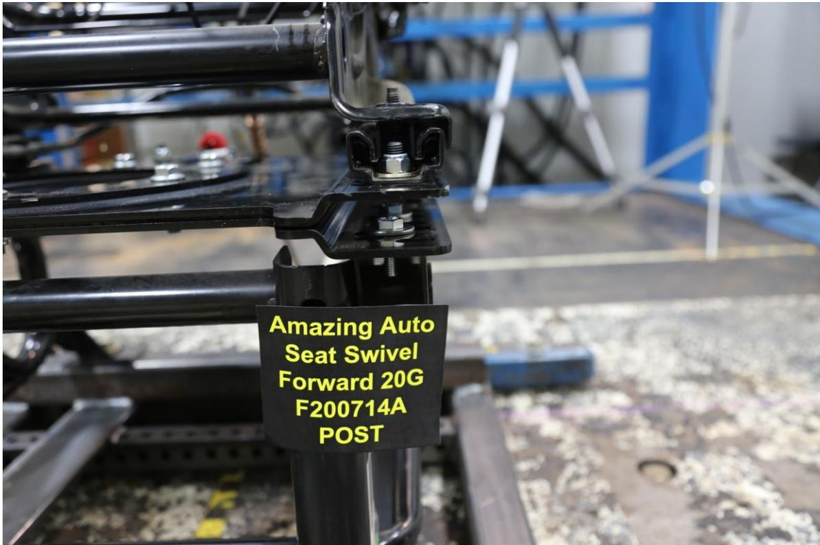
Figure 15 F200714A Post-Test Swivel Attachment View 2
