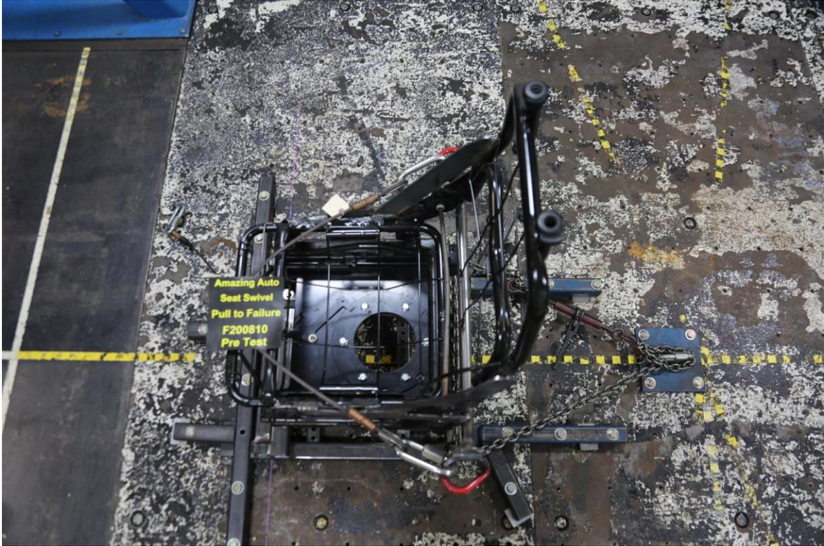
**Figure 47 Seat Base and Swivel Attachment to Bed Plate - Top View**
