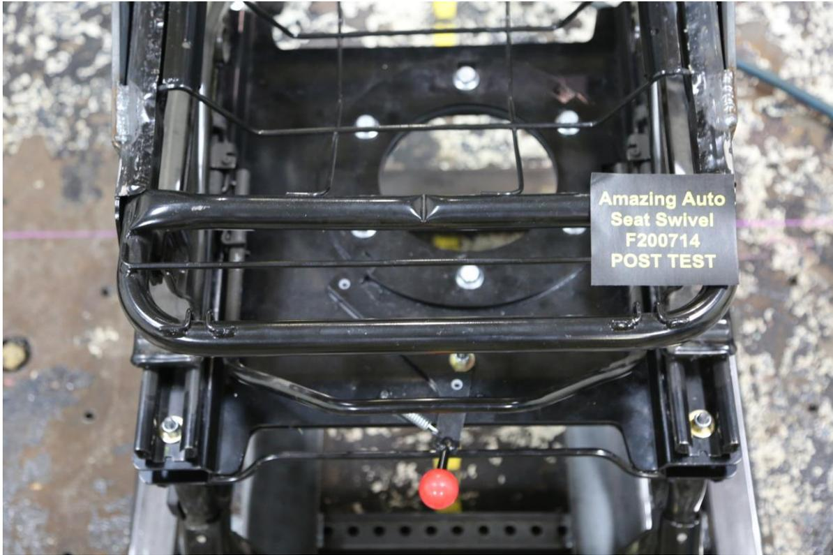
**Figure 43 Seat Frame to Swivel Front Attachment Bolts View**
