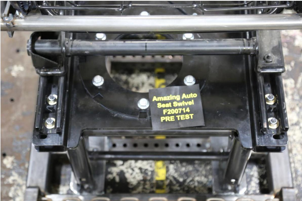
**Figure 4 Seat Frame Attachment Bolts to Swivel - Rear View**
