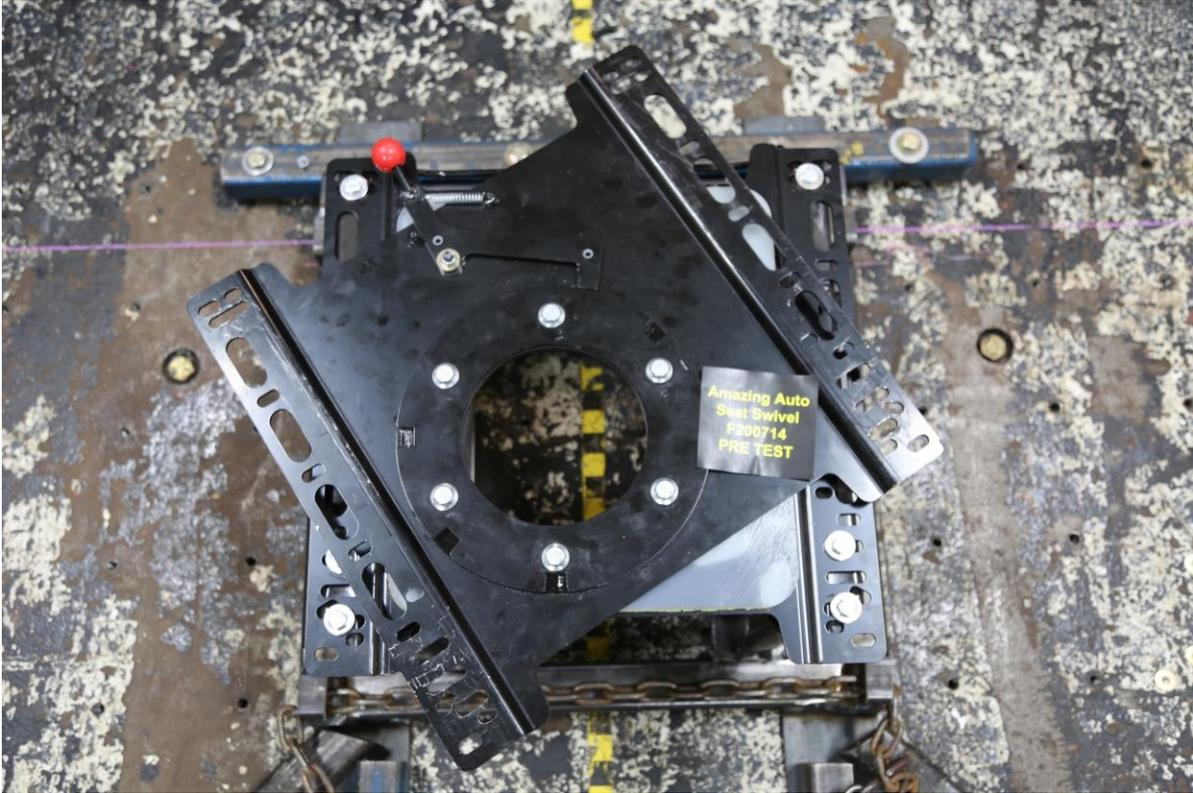
**Figure 3 Swivel Attachment Bolts to Seat Base - Top View**
