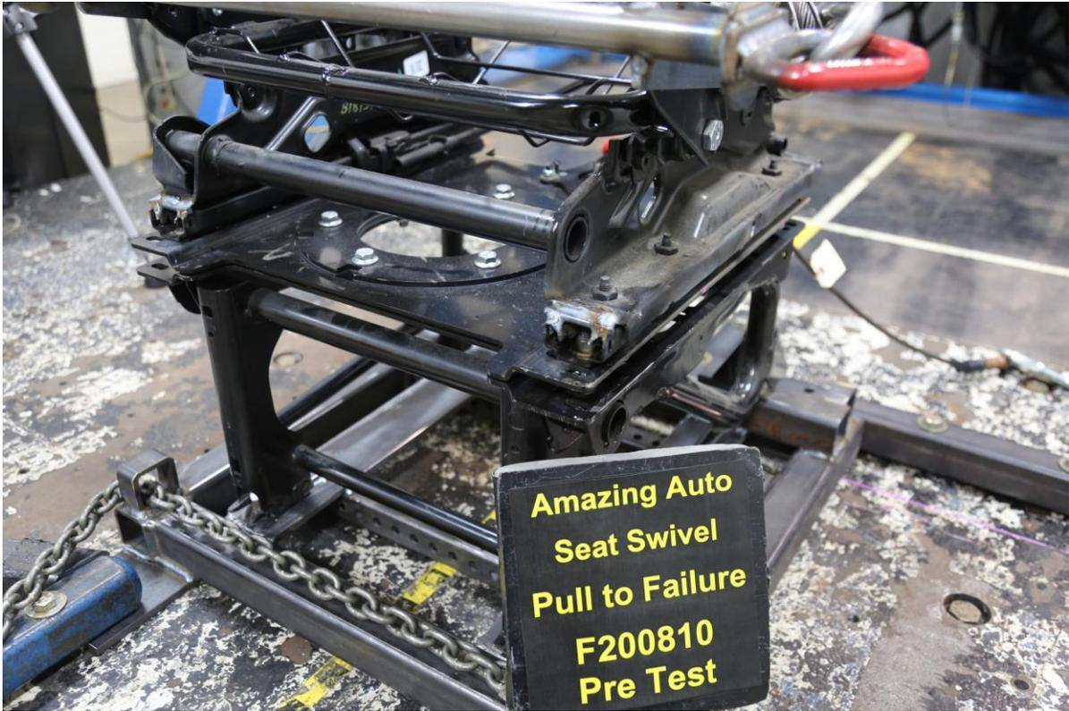
**Figure 49 Seat Frame Attachment Bolts to Swivel - Rear View**
