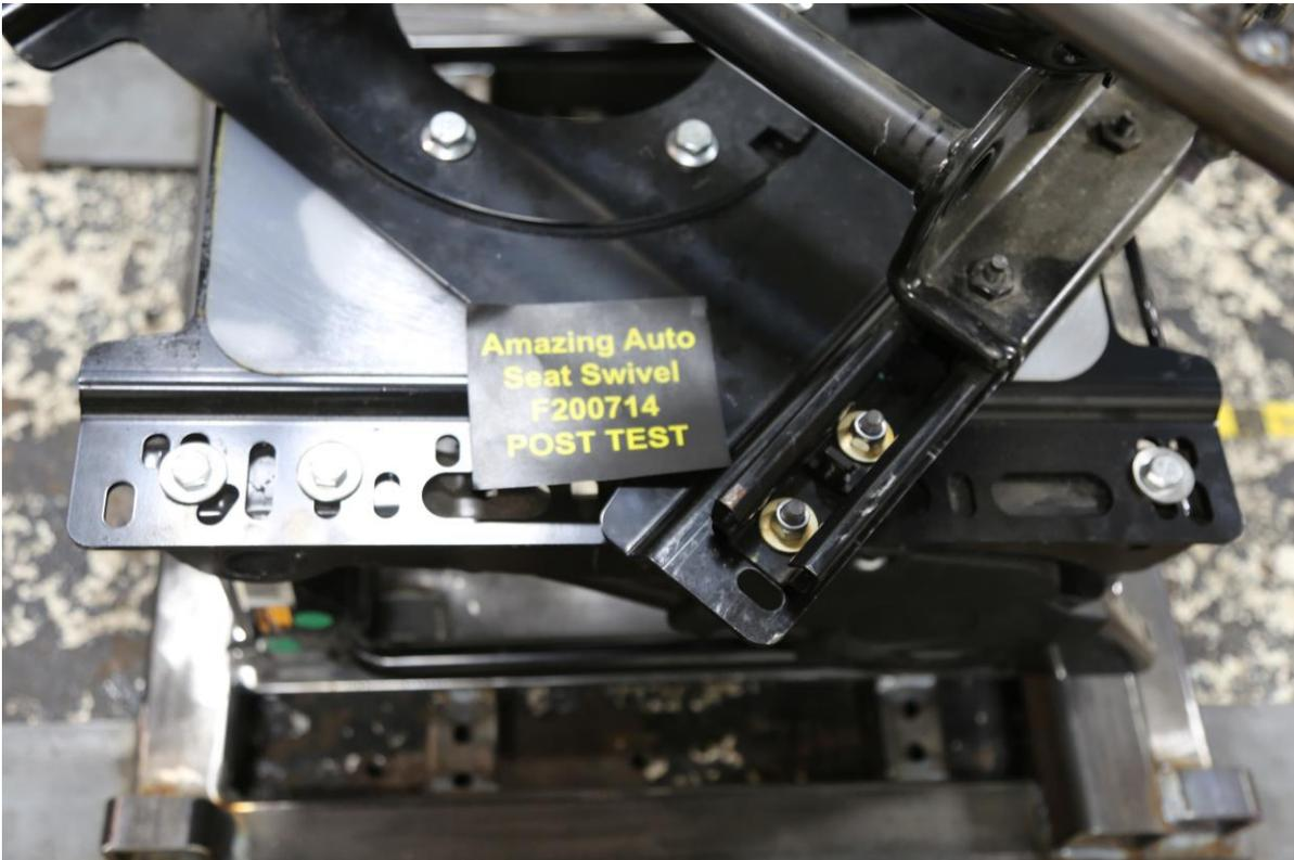
Figure 46 Swivel to Seat Base Right Side Attachment Bolts View
