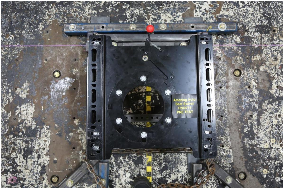
**Figure 2 Seat Base and Swivel Attachment to Bed Plate - Top View**
