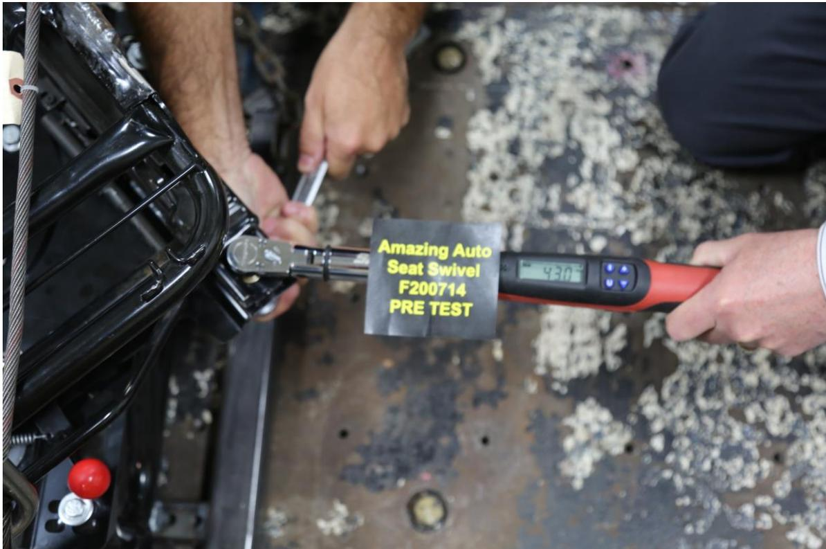
Figure 6 Swivel Attachment – Demonstrating Bolt Torque
