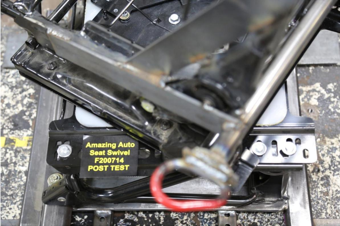
Figure 45 Swivel to Seat Base Left Side Attachment Bolts View
