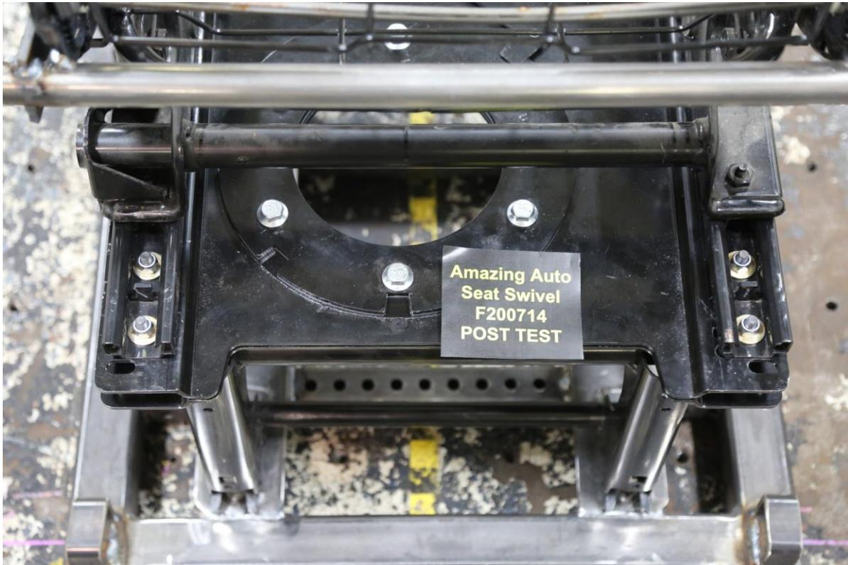
**Figure 44 Seat Frame to Swivel Rear Attachment Bolts View**
