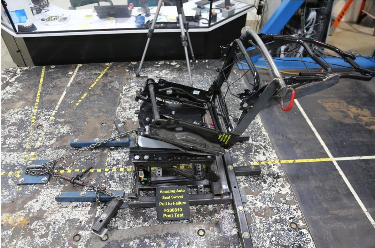
**Figure 64 F200810 Post-Test Right Side View**
