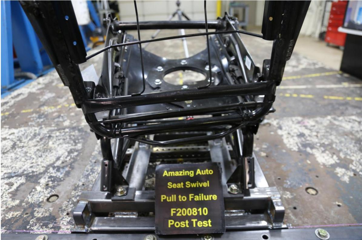
**Figure 52 F200810 Post-Test Front View**
