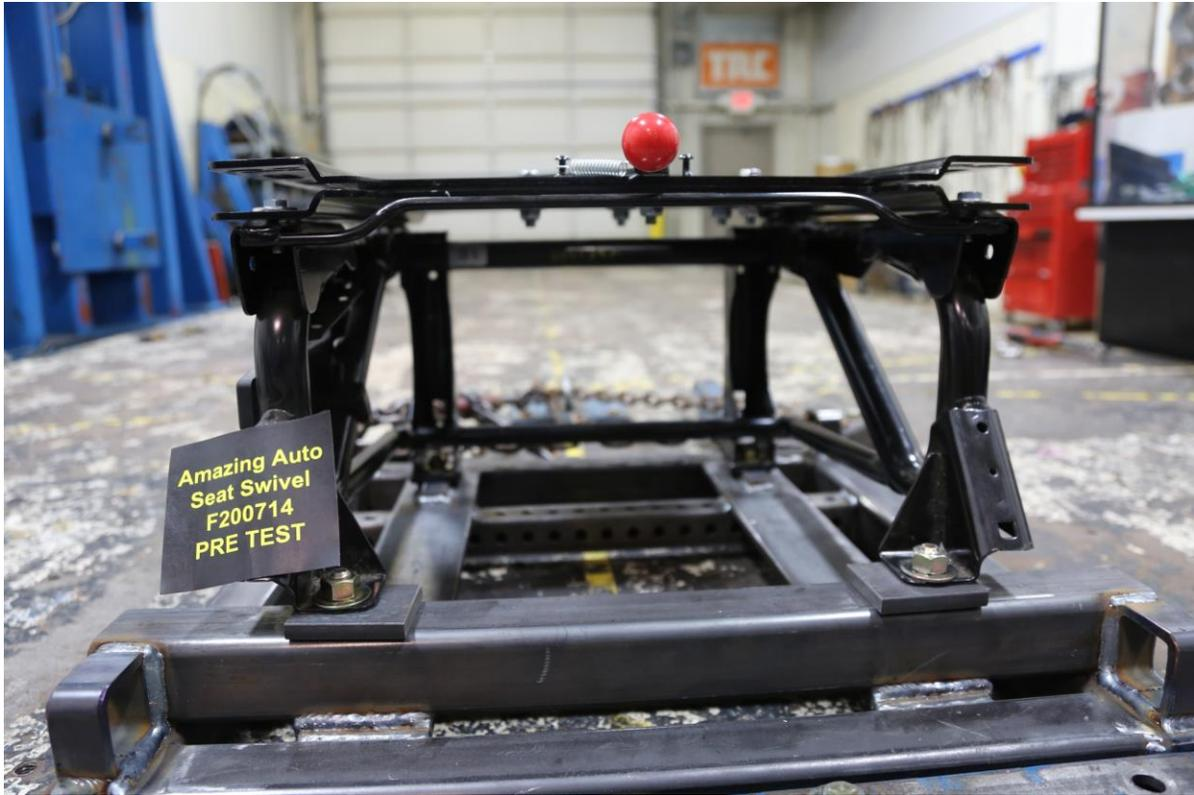
**Figure 1 Seat Base and Swivel Attachment to Bed Plate - Front View**
