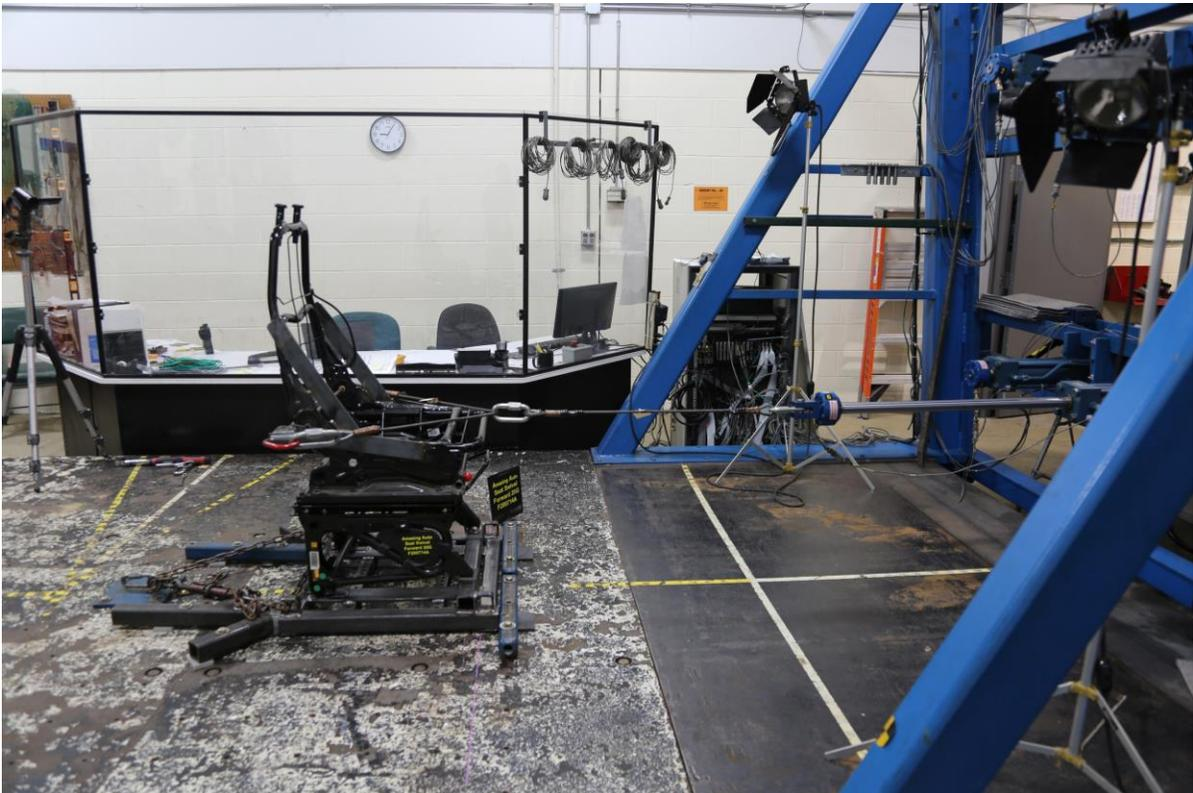
**Figure 17 F200714A Seat at Pre-Load Right Side View**
