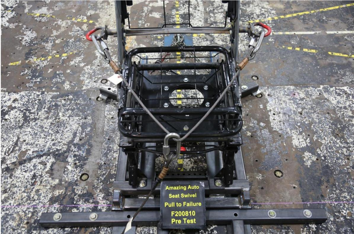
**Figure 48 Swivel Attachment Bolts to Seat Base - Top View**
