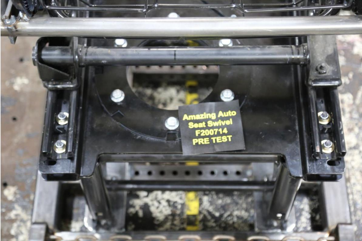
**Figure 13 F200714A Pre-Test Swivel Attachment View**
