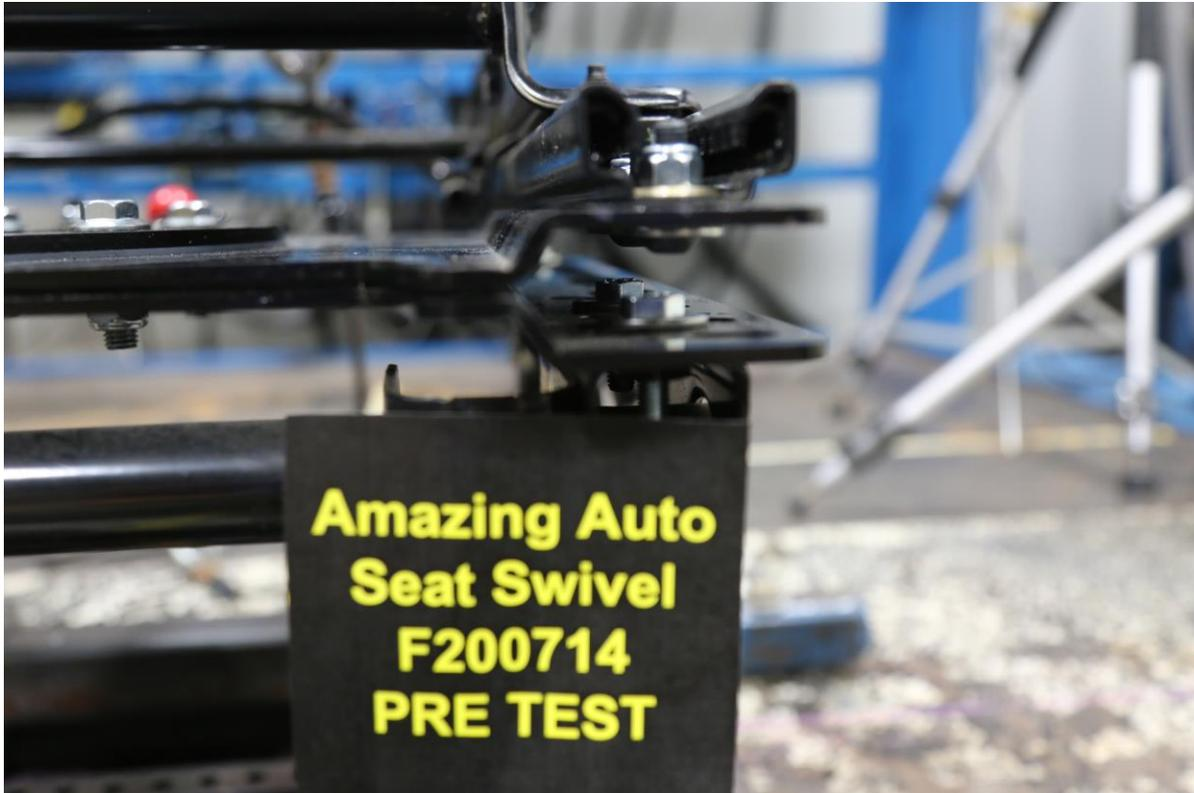
Figure 5 Seat Frame Attachment Bolts to Swivel - Front View
